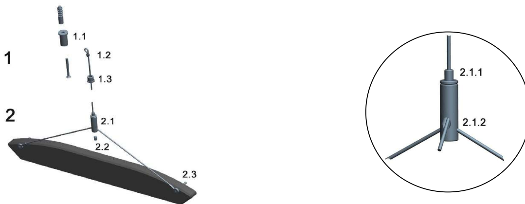
Fig. 2: Steel wire suspension aquafit 2 (art.-No. 80401)
